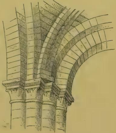
FIG. 166 BIS. — DÉTAIL DE LA PILE D'ANGLE
